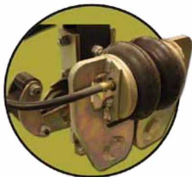
*Center Point's simple design cushions the RV against road shock by adding an air bag at the equalizer position between the leaf springs providing smooth, stable towing.*
