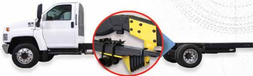
The E-Z Cruise™ rubber suspension system was designed to give the vehicle a smoother/more stable ride and improved anti-sway control, resulting in greater safety and added comfort for drivers and passengers alike.
