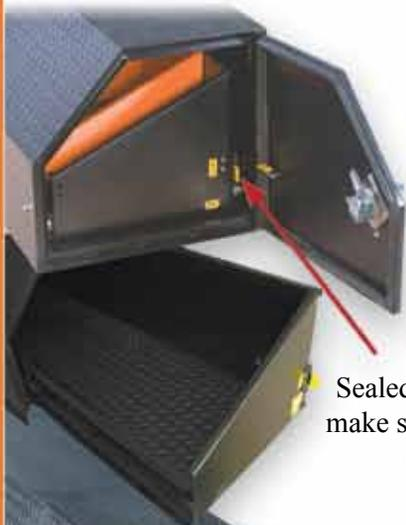
Sealed roller bearings make sliding in and out effortless.
